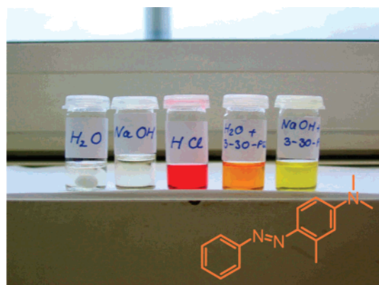
Figure 8. Solubilization of a hydrophobic azo dye (see inset) by polyelectrolyte brush 3-30-1a ; no solubilization occurs in pure \text{H}_2\text{O} and \text{NaOH} (left). \text{HCl} causes solubilization by protonation (middle, red). Addition of 3-30-1a to the \text{NaOH} solution results in a yellow solution (right), in which the dye is solubilized by the hydrophobic parts of the brush molecules. In aqueous solution, both solubilization mechanisms are present due to the brush's intrinsic acidity.
